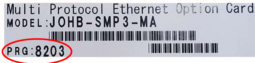
Fig. 2 Example of firmware version 8203 on the option card packaging
